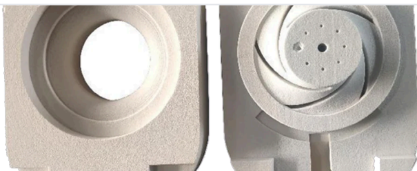
Impeller volute mold — printed as one piece, no pattern shop involved
