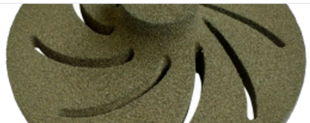
Pump impeller mold — curved passages that a corebox cannot reach
