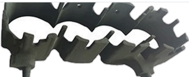
Engine block cores — a full core package printed in one build
